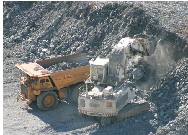
FIG 1 - The Liebherr 994 excavator monitored during the field study.
